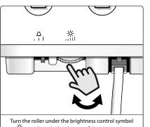
to adjust the brightness of the picture. Any adjustment to the left will reduce the brightness and any adjustment to the right will increase the brightness.
