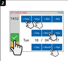
Use the buttons to adjust the date & time required then tap  $\checkmark$  to confirm.
