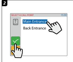
Select the door panel to connect to then tap  $\checkmark$  to open the communication.
