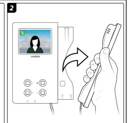
Pick up the handset. The display shows the video from the door panel.
