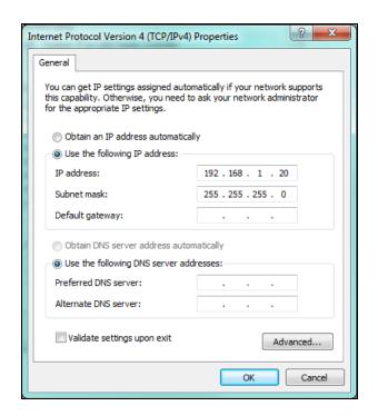
Reconfigure the EWS network configuration with the details shown below, and press 'Update and Reset'
