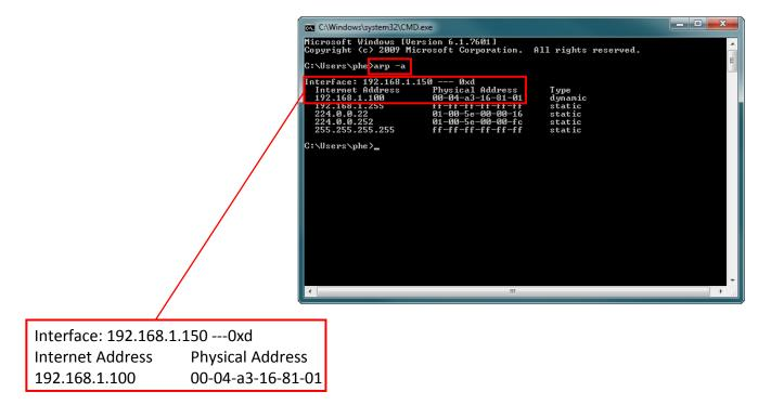
The 'Interface' is the current IP address of the PC/Laptop, the 'Internet Address' is the default IP address of the EWSi controller and the 'Physical Address' is the MAC address of the EWSi controller. The Physical address (as shown above) can be verified against the Serial No. and MAC address label on the EWSi controller itself.
