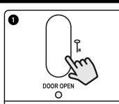
During a conversation, with the handset lifted, press the lock button <sup>0</sup>−π to operate the lock.
